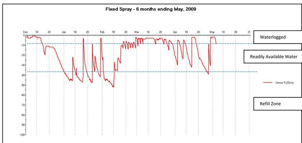
Fig 2: Soil moisture levels under sub-surface drip irrigation
